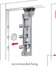
countersunk head wood screws Ø3,5x20 mm
