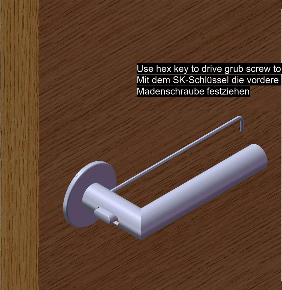
Use hex key to drive grub screw to fix spindle
