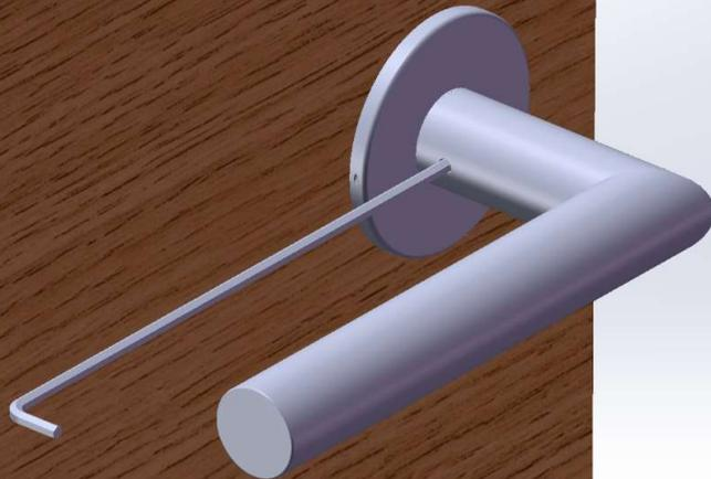
Keep the hex key in the hole and press the handle down to unlock.
