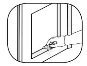
Smooth out any rough edges with sand paper or a file. Refer to the Quick Start Guide for fitting.
