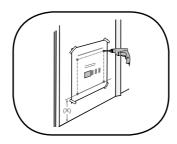
Position the cutting template base at belly height marked on door (X). Drill holes at corners as indicated.
