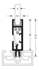
Integrated shelves lighting with hidden cable routing inside the frame side.
